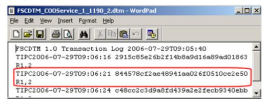
The color bordered part represents an entry for a transaction in the log file. The entry displays a transaction (T), which was initialized (I), prepared (P) and finally closed (C). Then the start time of the transaction is displayed followed by the global identification, the XID. In the line below the involved resources are mentioned. In this case these are the Fabasoft Folio COO Services with the instance numbers 1 and 2.
